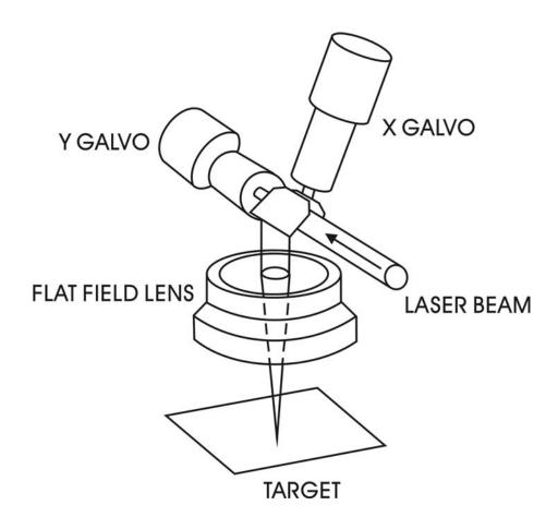
X and Y Galvanometric Scanners with a Flat Field Lens
