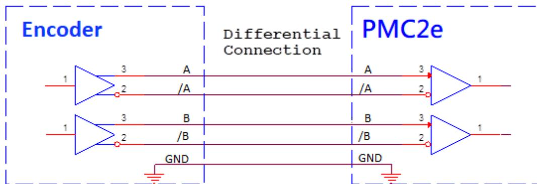
Note : Encoder GND should short to PMC2e GND.
