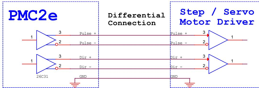
Note : Motor Servo GND should short to PMC2e GND.
